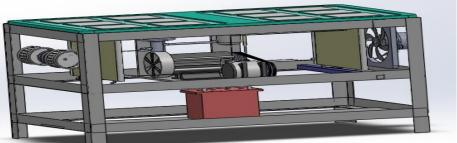
battery which let the motor rotates. The motor used here is the 1H.P DC motor. **Fig:-4 Solar A/c Panel and Motor**
