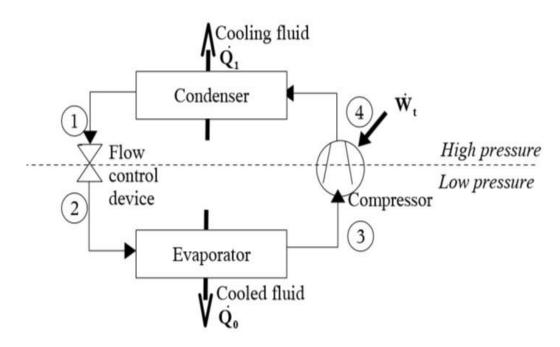
though a restriction, known as flow control device. The pressure of refrigerant decreases through the restriction. At a very low pressure that a small portion of the refrigerant vaporize into a gas. But in order to vaporize, it requires heat, thus cooling the mixture and results in a low temperature.
